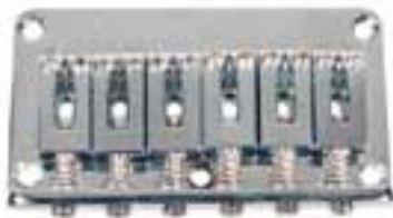
bridge-tailpiece, Stallion, pitch 10,5mm, strings through body
